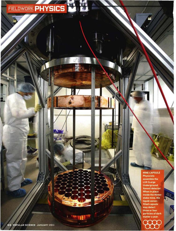
actually detect the dark matter so precision is essential. But the various parts were machined at different sites, and without that perfect seal, air and impurities could infiltrate the experiment, potentially compromising the results. As Tom Shutt, a physicist at Case Western Reserve University and the co-founder of the LUX project, explains, "We've been on pins and needles to know how tight this can will be."
